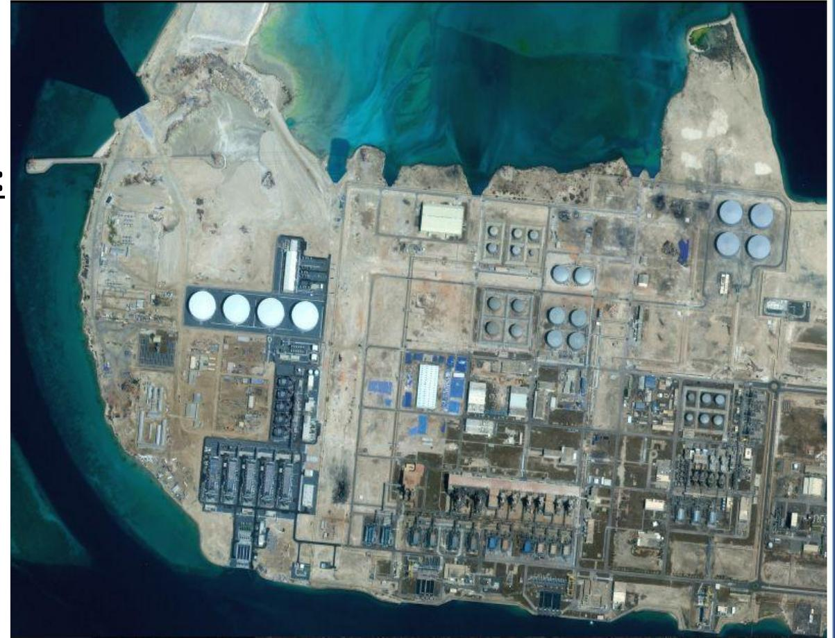
**UMM AL NAR WEST POWER & DESALINATION PLANT (UNITS 1 TO 6) 4x35.4 6x60 MW EXTRACTION CONDENSING TYPE TURBINES, 6X365 TONS/HR NATURAL GAS AND LIQUID FUEL FIRED BOILERS AT 60 BAR AND 480 C AND 6X4 MIGD DESALINATION PLANT**
